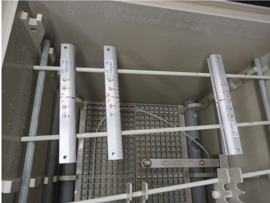
Figure 3: Test sample in the salt mist treatment device.
