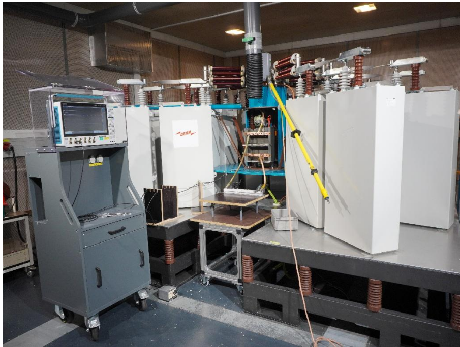
Figure 9: Electrical test – Overall view of the test set-up in the 50 kA (10/350 \mu s) Impulse Current Generator.
