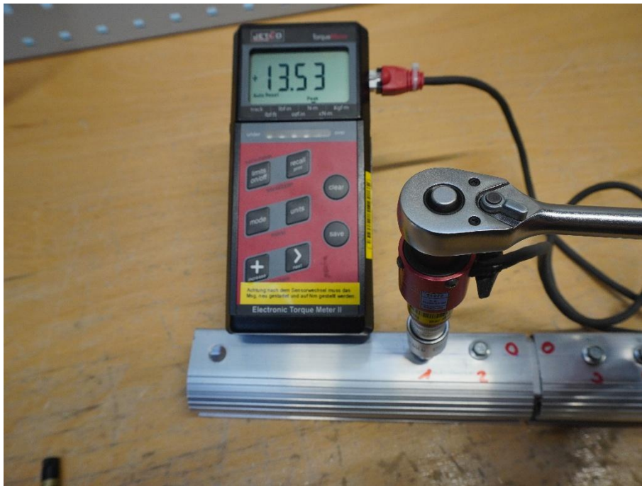
Figure 19: Measurement of torque – exemplary for all screws.
