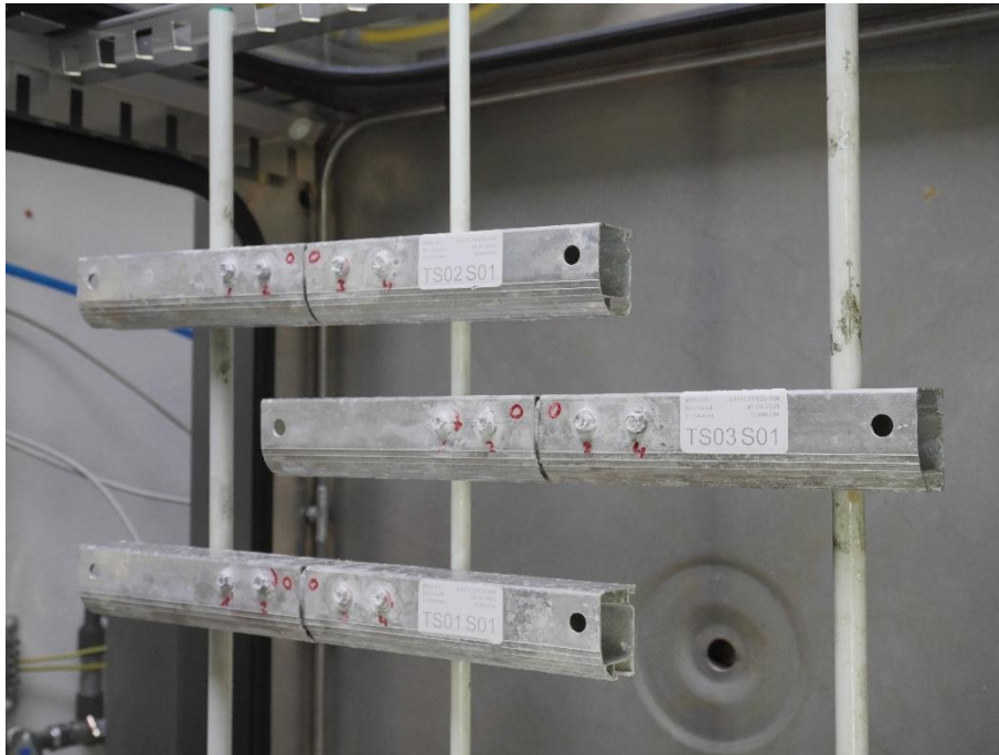
Figure 5: Test samples in the humid sulphurous atmosphere device.
