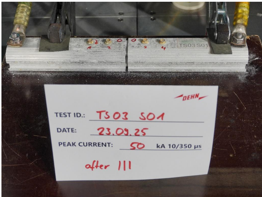
Figure 16: Test sample TS03 S01 after test with 3x 50 kA (10/350 \mu s).
