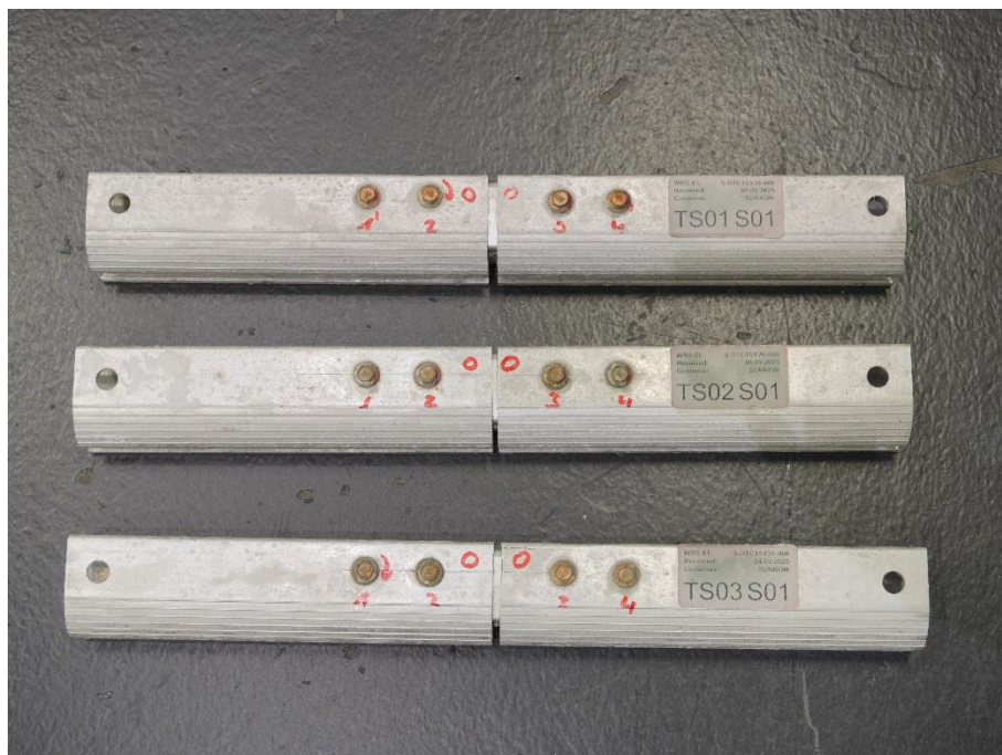
Figure 8: Test samples after the conditioning/ageing process.
